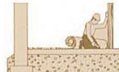
4. Remove floor covering
